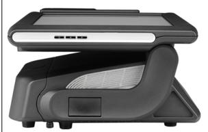
AL-9700 incorporates a virtually silent fan that is controlled according to the ambient temperature. The heavy-duty, all metal construction minimises the need for a fan but, because the CPU is so powerful, the fan is called into operation as and when necessary.
